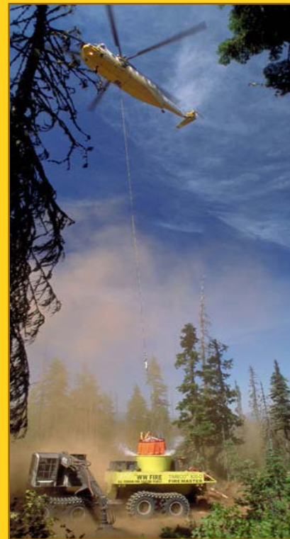
Helicopter aerial bucket refill of Super-skidgine tank
