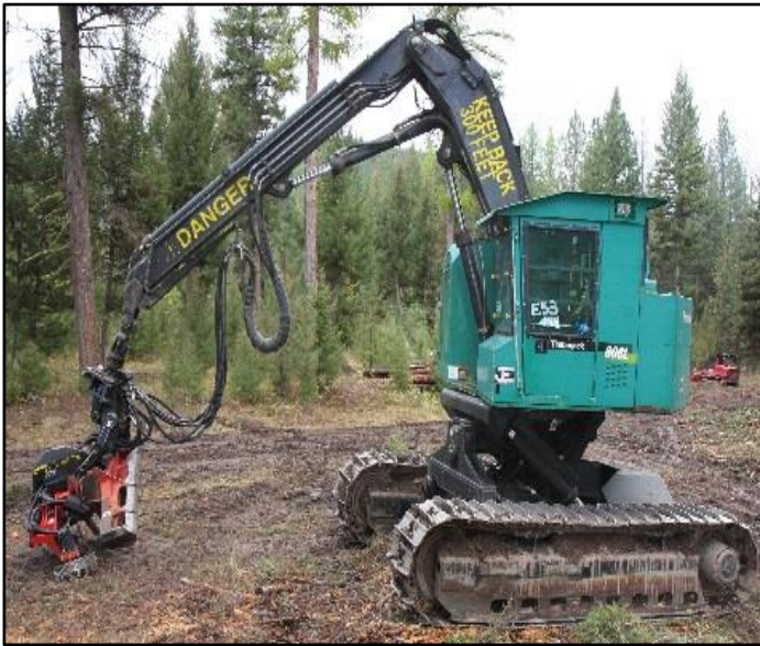
Reinforced cab on tracked harvester. Photo credit: JSteele
